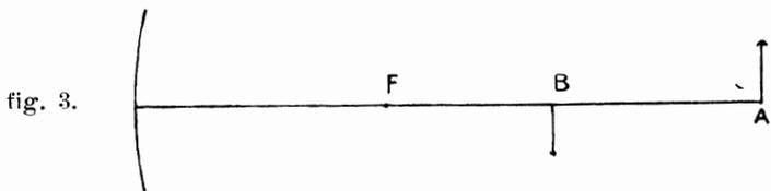
A catoptric telescope has the focal distance of  $f = 1.4$  yards. It is directed on a tree in the distance of 27.5 yards. Where will the picture be produced?
