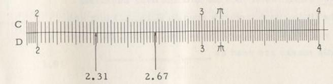
The number 2.31 is half-way between 2.30 and 2.32. You can place the hairline about half-way between two marks to read to one-hundredth; for example, 2.31. Half-way between the marks for 2.32 and 2.34 is the setting for \_\_\_\_\_.
