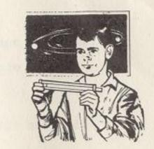
238. Notice the scale named A above the D scale. Place the hairline over 2 of the D scale. Then on the A scale you can read 4 or 2 x 2. Under 3 of D you can read 9 or 3 x 3 on A. The number 9 is the square of 3. The square of 3 can also be written 3<sup>2</sup>.
