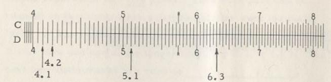
The spaces between 5 and 6, between 6 and 7, etc., are also separated into ten parts. Between 4 and 5, these marks can be read as 4.1, 4.2, 4.3, etc. Between 5 and 6 these marks can be read as \_\_\_\_, \_\_\_, etc.
