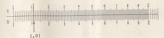
Now move the hairline over the first short mark to the right of 1.1. This is the mark for 1.11. Notice the space between 1.1 and 1.2 is separated into ten small parts. The little marks are read 1.11, 1.12, 1.13, \_\_\_\_, \_\_\_\_, etc.
