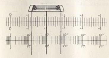
just above you find +2. The numbers for the X scale are the exponents for the D\* scale. The numeral +5 on X is just above 10 - on the D\* scale.
