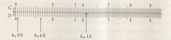
little mark between each of the marks for "tenths". Place the hairline on the mark for 4.60. The next little mark is for 4.65. The little marks are "counted by five hundredths". The little mark between 4.30 and 4.40 is the mark for \_\_\_\_.
