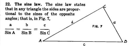
This law can be used to obtain the unknown parts in a triangle (right or oblique) with a single setting of the slide when two angles and a side are known.
