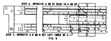
The above example illustrates the fundamental property of CF and DF, namely: When the slide is in any position, with a number x on D appearing opposite a number y on C, then this same number x appears also on DF opposite y on CF. If the reading is off scale on C-D it may be found on CF-DF.
