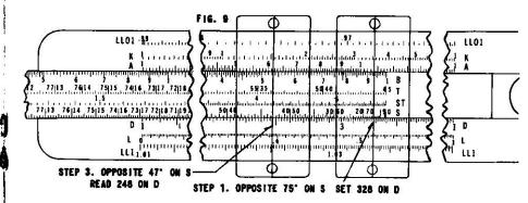
23. The tangent of an angle. The T scale gives the tangents and cotangents of angles between 5.71° and 84.29°.
