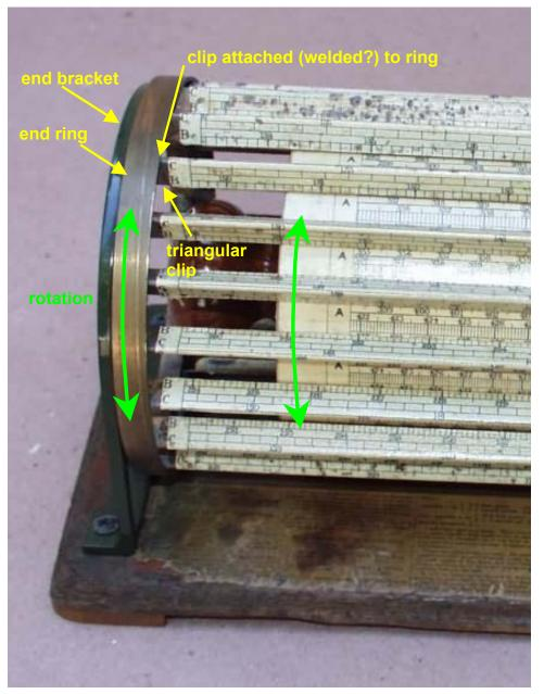
Figure 2 The rotating envelope mechanism.
