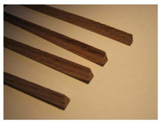
Figure 5 Triangular bars 3/8 x 1/4 x 3/8.
