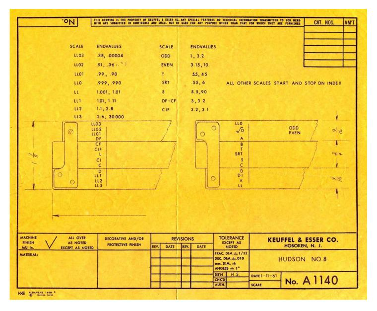
FIGURE 6. K&E specification sheet for Hudson 8.
