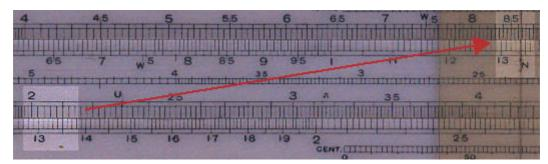
For most rules (i.e. ones with the special scales) the calculations of motor efficiency are simple mirror of the calculations for dynamo efficiency. However, for the Unique and others with gauge marks, the procedure is different.
