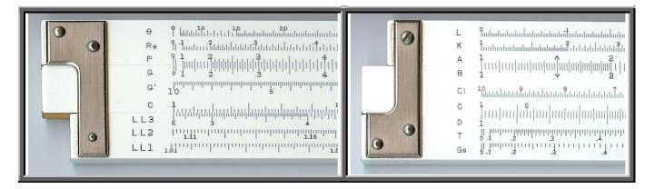
To obtain hyperbolic values of an argument x the Ge, T, P, Q and Q' scales where employed. Although the uses of the special scales on the 153 are not particularly intuitive they were, by and large useful in vector calculations. After some practice, the Ge scale provided very easy way to calculation of at least Sinh and Tanh values without the need for hyperbolic scales.
