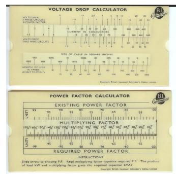
BICC PF and Voltage Drop Rules Note: BICC is an acronym for British Insulated Callender's Cables
