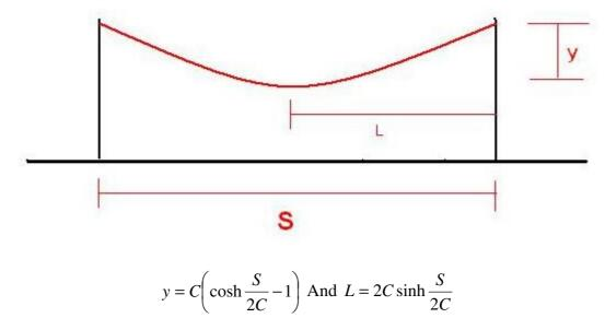
S is the span, s equals the sag, L is the length to the point of sag and C is a constant. Again, *hyperbolic functions* would have been an advantage.
