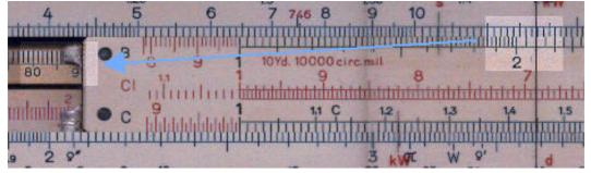
As a check, 21.0 multiplied by 0.746 is 15.67 and 13.6 / 15.67 is 86.2. As you can see it is not a complicated calculation, and personally I found it much easier to perform than to remember the actual scale settings. And as one usually needs to convert HP into watts for other calculations it was to some advantage to perform the calculation this way.
