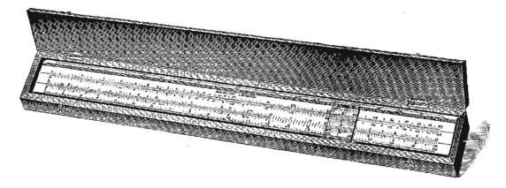
700 W. H. Harling's 20-inch SLIDE RULE, standard pattern, made of well-seasoned mahogany, faced with white celluloid, adjustable friction slide, full view glass cursor, graduated with the following scales:
