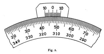
Figure 2 represents a scale and vernier very commonly met with, and which is largely applied to Protractors, as shown in Fig. 3, which is a  $5\frac{1}{2}$ inch Circular German Silver Protractor with a revoluble arm and vernier.
