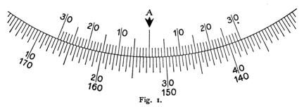
WE CONCLUDE these articles on Verniers by presenting those usually employed in connection with the graduations of the horizontal and vertical limbs of an Engineer's Transit. Clear and distinct graduations and well-combined verniers are in such instruments of great importance, and as the least count or reading can be obtained by different combinations of scale and vernier, it is essential that the one affording the greatest facilities for accurate reading should be selected.
