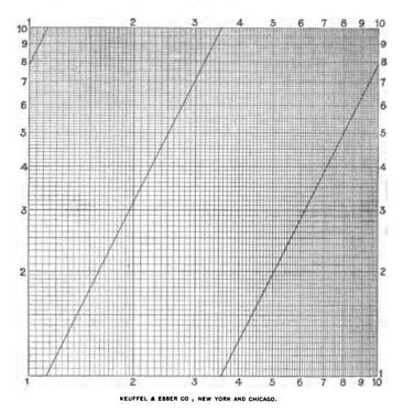
The above figure represents a sheet of cross-section paper in which the distances or spaces between the consecutive lines, instead of being all equal, or similar to those of a scale of equal parts, are logarithmic ones, the same as those of an ordinary slide rule.
