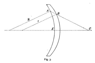
as shown in Fig. 3, where R is the radius of the near surface of the lens, and r the radius of the off surface, the lines R and r being drawn parallel to each other. A straight line is then drawn through the points A and B on the surfaces of the lens and extended to C on its axis. The point C, so found, is the optical centre of the lens, and the distance C E is its distance from the near surface of the lens as found by formula (7).
