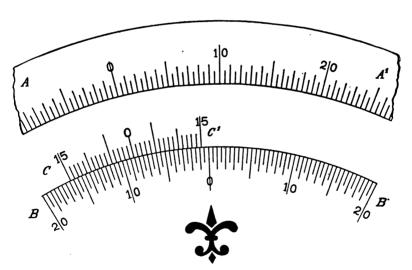
A VERNIER SOMETIMES met with is that shown in above figure which represents the general arrangement of a double vernier, as applied to the latest and most approved form of Transits and Surveyors' Compasses for the purpose of setting off the magnetic declination. In the figure the scale  $AA^1$  is a portion of the compass graduated circle,  $BB^1$  is a declination arc of 40 degrees, and  $CC^1$  is the vernier reading into the same.
