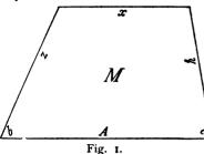
In figure 1, let b and c be the known angles, and let a be the sum of these angles subtracted from 180°. We then have for the length of the fourth side
