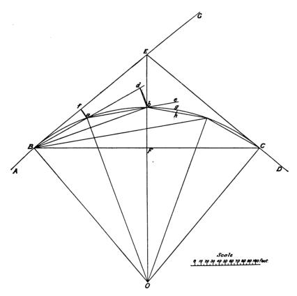
RAILROAD CURVES are designated by the angles which are subtended by a uniform chord too feet long, as a one-degree, two-degree curve, etc.
