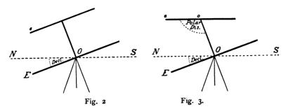
2. Level the solar telescope by means of its attached level, taking care that it has been previously brought exactly into the vertical plane of the transit telescope, as shown in Fig. 3. The angle  $O \circ e$  is then the polar distance of the sun, or the co-declination = SP of the astronomical triangle,  $= 90^{\circ} + 20^{\circ} = 110^{\circ}$ .
