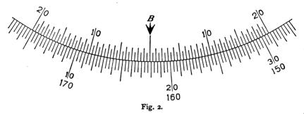
This is a double direct vernier similar to Fig. 1, but with finer divisions; it also reads from the centre to the right and to the left, according to the direction followed on the horizontal limb. The limb is graduated to thirds of a degree or 20 minutes, while each scale of the vernier is divided into 40 equal parts, and 40 vernier divisions correspond to 39 limb divisions, thus giving a least count or reading of 20 minutes or 1200 seconds  $\div$  40 = 30 seconds.
