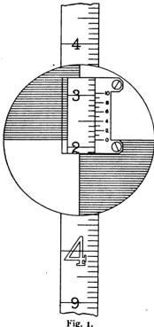
the rod. In the case of the architect's rod, the main divisions are feet, inches and eighths of an inch, while 8 divisions of the vernier correspond to 7 divisions of the rod or 7 ths of an inch, so that the least count is 1/44 th inch. We have already explained the principles of the vernier (Vol. I, p. 28,) so shall not refer to them here more than to explain how to take a reading with the different verniers we are about to describe.
