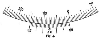
Fig. 4 represents a portion of the vertical limb or arc of an Engineer's Transit. As in Fig. 3, the space usually available for the vernier is very limited, so that a double folded vernier is indispensable; its main features are similar to those of Fig. 3, and the method of reading also the same.
