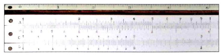
Figure 4.6.1.1.L: Left part of the front of the Rosenthal system from Dietzgen (prototype). Otto van Poelje collection
