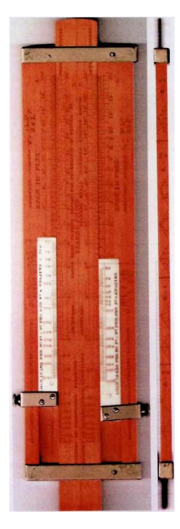
The front has 10 scales; the reverse (not shown) has 6 scales and a table. Despite the many scales and supporting texts, the staff is very clearly designed.
