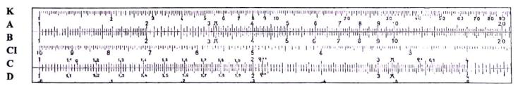
Figure 4.2.4.9: Left part of the front of the Rietz system
