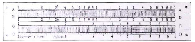
Figure 4.3.6.3: System Simplex pocket slide rule with rivets. IJzebrand Schuitema collection
