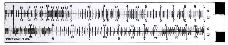
Figure 4.6.1.1.5.R: Right part of the front of the Rosenthal system from Dietzgen. Rodger Shepherd collection
