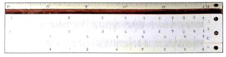
Figure 4.6.1.1.R: Right part of the front of the Rosenthal system by Dietzgen (prototype). Otto van Poelje Collection
