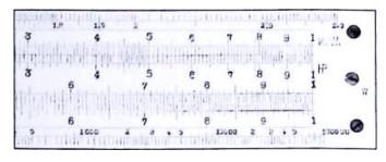
Figure 3.6.I.5.R: Right part of Schweth's Electro slide rule
