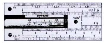
Figure 3.6.1.5.L: Left part of Schweth's Electro slide rule
