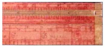
Figure 6.11.3: Section of the Coggeshall system
