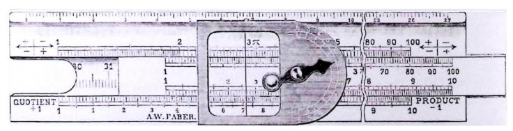
Figure 3.8.1.1: Direct marking of the number of digits by means of inscriptions and marks
