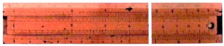
Figure 3.4.6: Front of the Soho system by Tavernier-Gravet with the bevelled ruler scale and handling button
