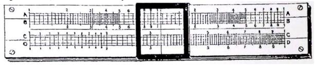
Figure 4.3.6.1: 1903 system Simplex pocket slide rule with screws. Journal of Surveying
