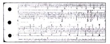
Figure 4.4.4: Slide rule System Rietz
