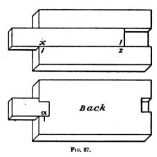
If the slide is inverted we can use the T scale in conjunction with the right-hand mark at the back of the ruler. Pulling out the inverted slide to the right until  $\alpha$  on the T scale is opposite the right-hand mark at the back of the ruler, we read tan a on the bottom scale of the ruler opposite the end of the slide and  $\tan^2\alpha$  (or on adding unity to the reading  $\tan^2\alpha + 1$ , which is  $\sec^2\alpha$ ) on the top scale of the ruler above the same end of the slide.
