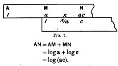
Note that this "setting" of the slide gives a table for multiplication by a, for opposite each number on the slide is a times that number on the ruler.
