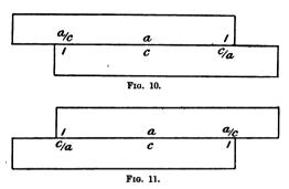
Returning to Fig. 9, where a on the slide is opposite c on the ruler, we have, if the whole length of the slide represents log 10,
