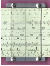
2.6mm thick Aluminum Stock No Serial Numbers Plain Flat Lenses Grooved Stock
