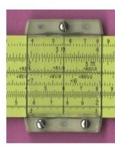
Nylon Cursor Bars, Grooved Convex Lens
