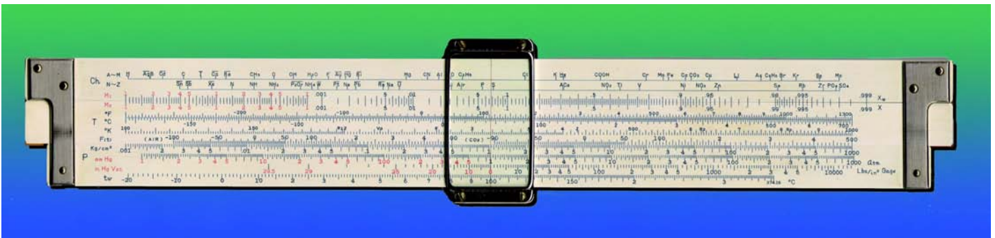
HEMMI 257, 25 CM SCALES, CELLULOID ON BAMBOO CORE, DUPLEX, JAPAN. FRONT AND BACK VIEWS
