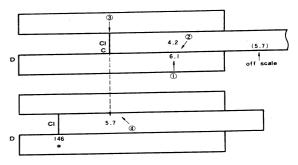
The above operations mean that the problem of  $a \times b \times c = x$  is solved in such a manner as  $a \times b = y$  and  $y \times c = x$ . Therefore, the third number 5.7 is to be set on the CI scale basing on the principle of multiplication and division of two numbers. If the third operation is a division as the problem of Ex. 4.6, set the third number on the C scale.
