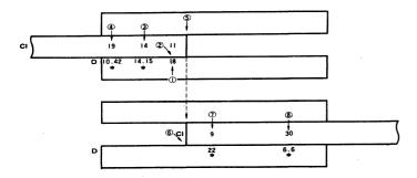
In this exercise 9 and 30 run "off scale". In this case it is more efficient to calculate the figures (19 and 14) which are inside the rule before interchanging the indices.
