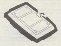
The exposed metal contacts on the battery pack are the battery terminals. Care should always be taken to prevent any metal object from coming into contact with the terminals and shorting the batteries.
